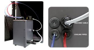
**4.** Position the water bath in front of the soundproof box upon the final site. Connect the Bioruptor<sup>®</sup> water bath to the Bioruptor<sup>®</sup> Water Cooler with the red and blue tubes by inserting them in the appropriate connectors.
