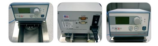
Fill the tank of the circulator with 4.5 litres of water. Distilled water should be used in order to minimize the proliferation of bacteria.
