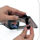
**3.** Place the two black plastic connectors on the motorized lid. The connectors can be placed into one or the other hole of the motorized lid.
